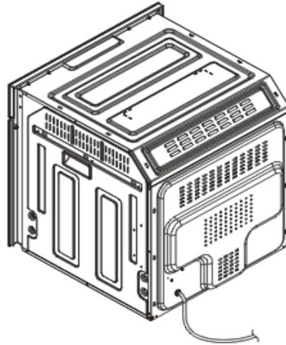
The connection cable must be secured in a strain-relief clamp.
