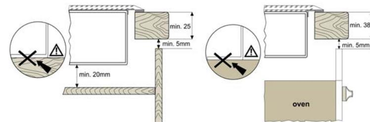
WARNING: Under no circumstances should the cooktop be installed directly onto a shelf.
